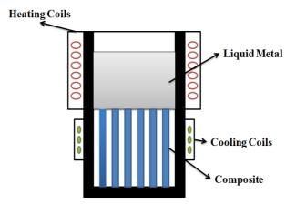
Figure 2.6: Process of in Situ Synthesis
