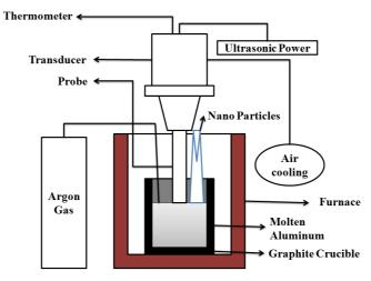
Figure 2.8: Design of Ultrasonic Assisted Casting Process
