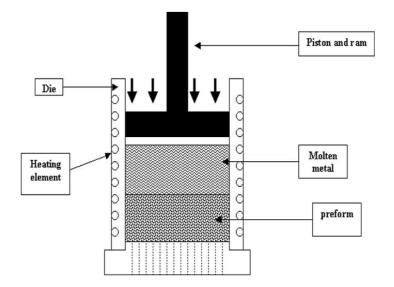
Figure 2.3: Schematic Diagram of the Squeeze Casting Apparatus [33]
