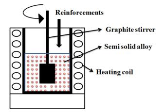
Figure 2.2: Design Setup of Compo Casting
