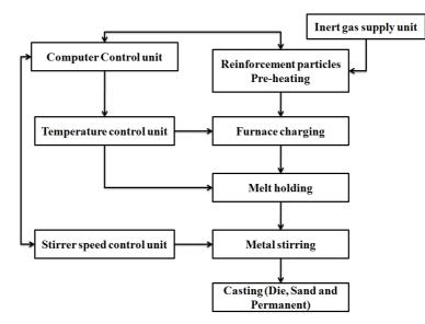
Figure 2.1.1: Flow Chart of Stir Casting Process
