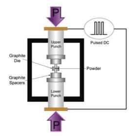
Figure 2.10: Schematic of the Spark Plasma Sintering Apparatus [76]
